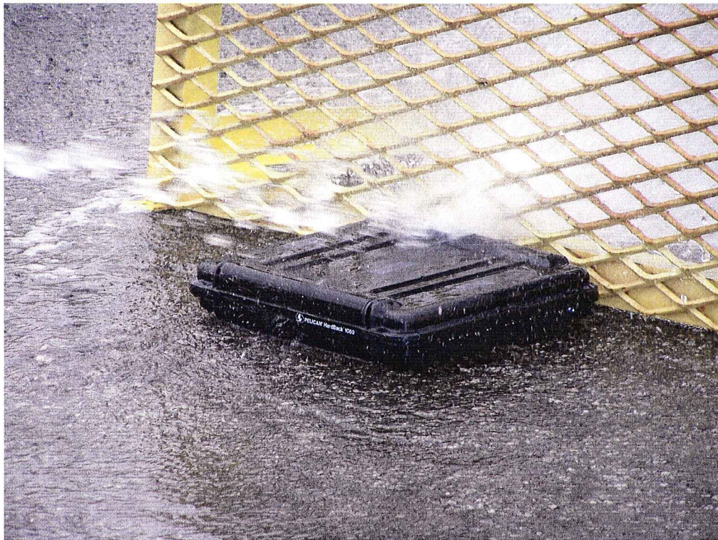
Photograph 4 Rain Intrusion Test Setup
